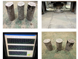
Strength Test : KS F 2422
